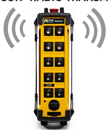
RaCon transmitter models ending with MI, EC and SP have a vibration alarm as standard. When the battery is running low, the alarm goes off and the transmitter starts vibrating. Vibration alarms are optional in some models.
