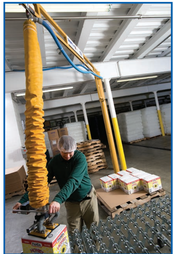
A worker stacks boxes of packaged food onto a pallet using a Spanco 150-Pound Capacity Freestanding Workstation Jib Crane with a vacuum attachment.
