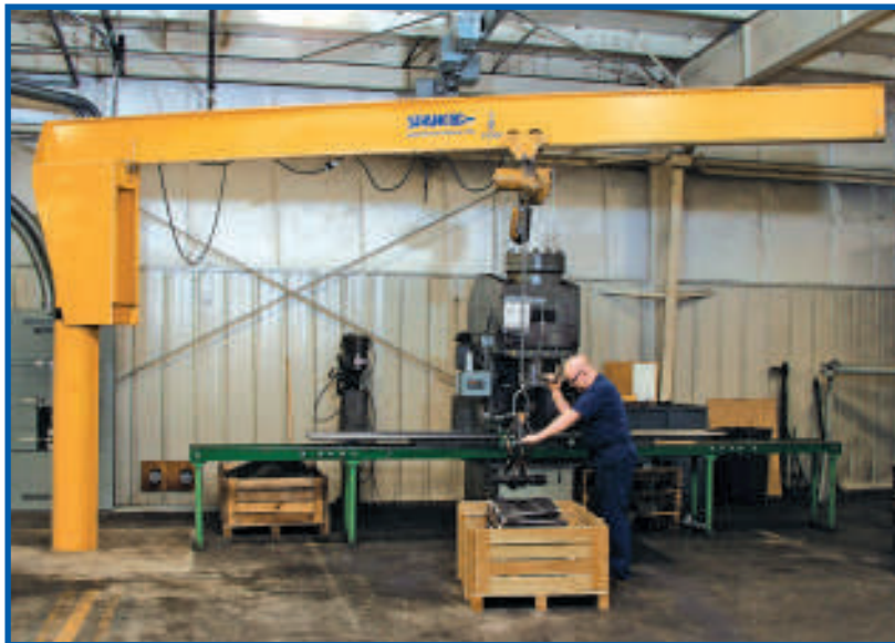
A worker lifts parts into a metalworking machine using a Spanco 1/2-Ton 101-Series Freestanding Jib Crane.
