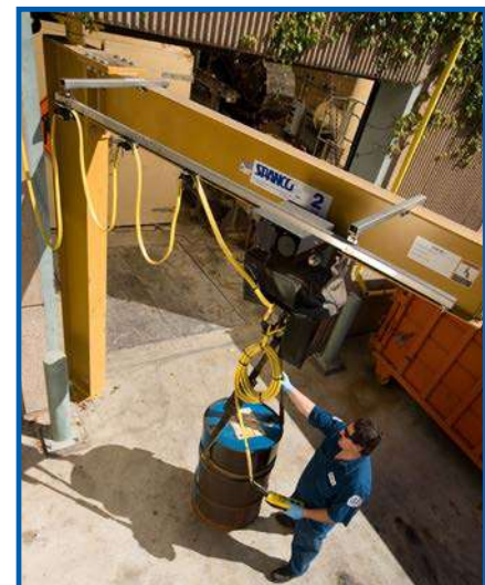
Spanco 201-Series Mast-Style Drop-Cantilever Jib Cranes are similar to the 200-Series Full-Cantilever Jib Cranes, with the addition of side-plate connections to "drop mount" the boom permanently at a specified height on the mast. This design allows for clearance from overhead obstructions located below the top of the mast.
