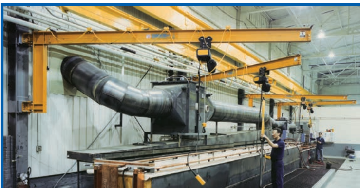
At this plant, four Spanco ¼-Ton 300-Series Wall-Mounted Jib Cranes load and unload materials from a production bench. They can also transfer goods to adjacent cranes' coverage areas.
